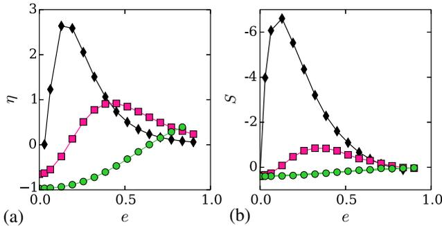
FIG. 4 (color online). Numerical simulations of 2D metabeams of 5.4% aspect ratio ( $\varepsilon_b = -0.0096$ ) and  $6 \times 111$  holes for the nonlinearity  $\eta$  (a) and postbuckling slope  $S$  (b) vs  $e$  for  $\ell = 0.13$  (black diamonds),  $\ell = 0.23$  (pink squares), and  $\ell = 0.42$  (green circles). See Ref. [30] for movies.
