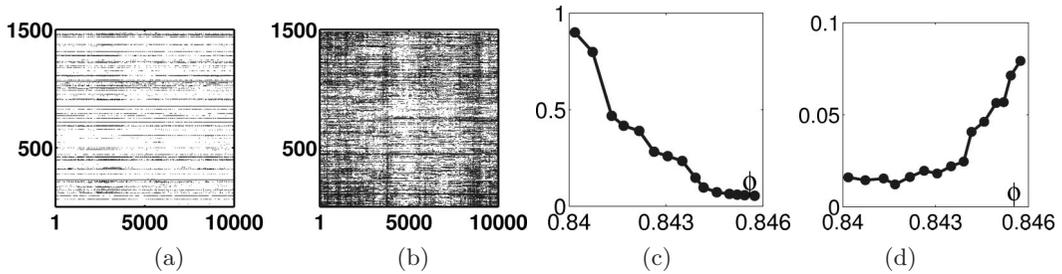
Fig. 3. Typology of rattling particles. (a) Label of the rattling grains vs time for the highest packing fraction explored  $\phi = 0.845$ . (b) Same for the loosest one  $\phi = 0.84$ . (c) Fraction of particles which have rattled at least once vs the packing fraction. (d) Averaged fraction of time spent rattling by rattlers vs the packing fraction.
