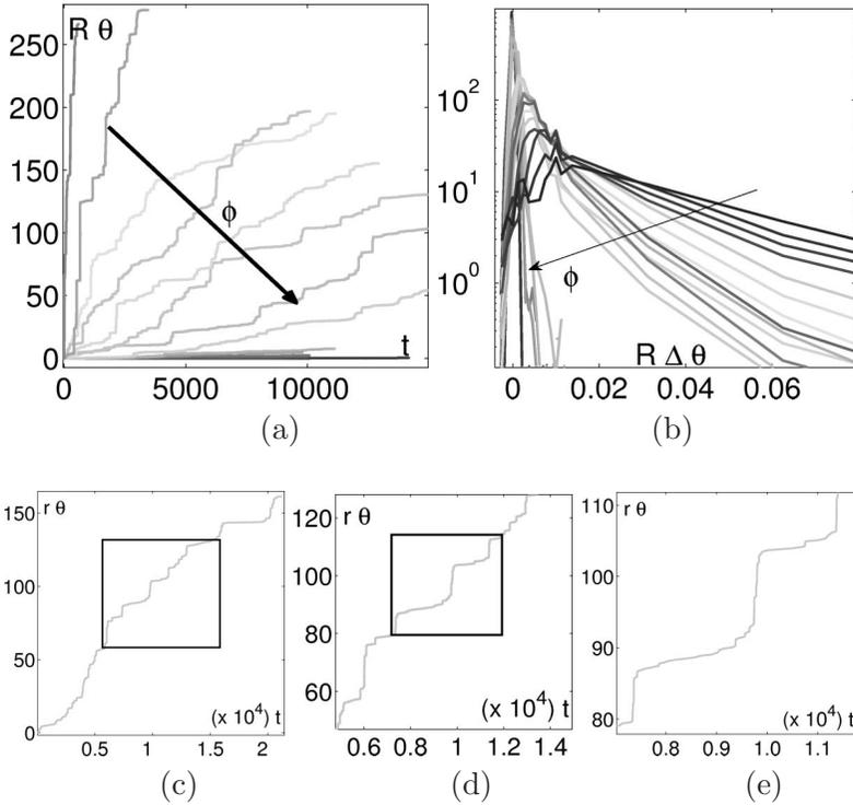
Fig. 4. (Color online) (a) Angular motion of the rheometer for several packing fractions, from  $\phi = 0.8385$  (red) to  $\phi = 0.8416$  (blue), at constant torque ( $T = 0.138$ ). (b) Distribution of instantaneous displacements of the rheometer  $R\Delta\theta$  for the same parameters. (c,d,e) Two levels of magnification on the angular motion of the rheometer for a surface fraction close to Jamming, and a torque  $T = 0.138$ .
